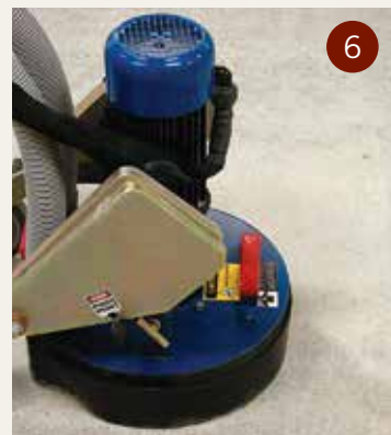
Diamond grinding: for horizontal surfaces.
